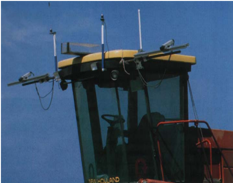
Aerials and cameras mounted on the cab roof collect data and images for the automatic guidance system on the New Holland NH2550 self-propelled swather.
