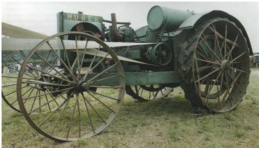
The Waterloo Boy tractors were not alone in retaining a steel-frame structure well into the 1920s.
