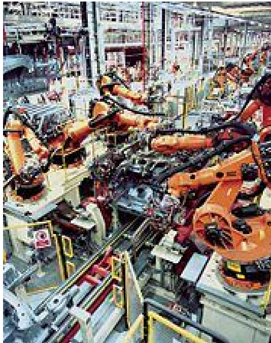
Industrial robots engaged in vehicle underbody assembly
